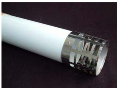
Fig.no.15 Pipe for flue gas exhaust or the air inlet with an outfall through a wall Ø 80 mm (Ø □100 mm), pressure loss: 10 Pa
