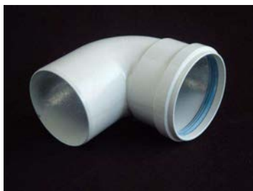
Fig.no.13 90° elbow Ø 80 mm (Ø □100 mm) Pressure loss: 14 Pa
