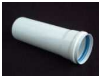
Fig.no.14 Separate extension pipe horizontal Ø 80 mm (Ø □100 mm), pressure loss: 3 Pa
